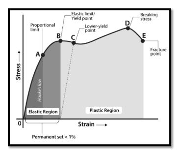
From the curve, we see that from point O to B, the region is an elastic region. After that, the plastic deformation starts. The point A in the curve shows the limit of proportionality. For this curve, we can write the value of Modulus of Elasticity (E) is equal to the slope of Stress-strain curve up to A.
