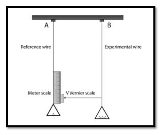
Take two identical straight wires (same length and equal radius) A and B. Now fix its end from a fixed, rigid support. The wire A is the reference wire, and it carries a millimetre main scale M and a pan to place weight. The wire B is the experimental wire. It also carries a pan in which known weights are placed. At the bottom of the wire, B attaches a vernier scale V.
