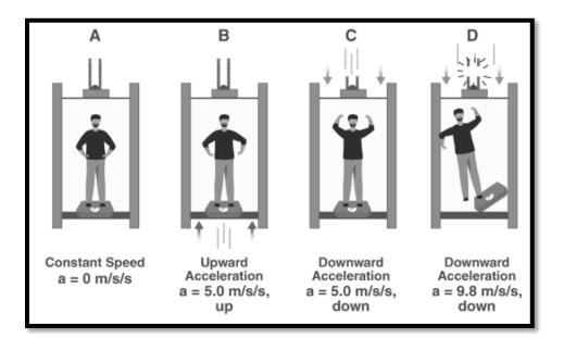
In the diagram, Otis's 80-kg is traveling with constant speed (A), accelerating upward (B), accelerating downward (C), and free-falling (D) after the elevator cable snaps. The normal force is greater than the force of gravity when the elevator accelerates upwards (B). And it is lesser than the force of gravity where there is a downward acceleration (C and D) and is equal to the force of gravity when there is no acceleration.
