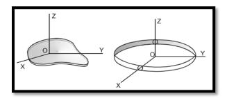
According to this theorem the moment of inertia of a lamina about an axis passing through its axis and perpendicular to its plane is equal to the sum of moment of inertia about the two mutually perpendicular axis in the plane of lamina. The normal axis OZ must pass through the point intersection of two mutually perpendicular axes OX and OY
