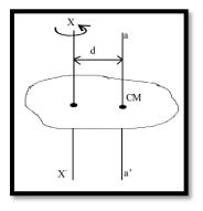
According to this theorem, the moment of inertia of a body about any axis is equal to the sum of moment of inertia about an axis passing through its centre of gravity and parallel to given axis and product of its mass and square of distance between the center of gravity and the axis of rotation.
