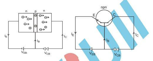
As one electron reaches the collector, it flows to the +ve terminal of  $V_{CB}$ , At the same time one electron flows from negative terminal of  $V_{CB}$  to +ve terminal of  $V_{EB}$  & one electron flows from -ve terminal of  $V_{EB}$  to emitter. Thus, in n-p-n transistor, the current is carried inside the transistor as well as in external circuit by electron. So the direction of conventional current is opposite to direction of flow of electrons.
