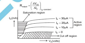
Output characteristics of a transistor in common - emitter configuration are divided into three regions :
