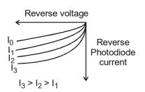
**Uses :** (i) In photo detecton for optical signals. (iii) They are used as light operated switches
