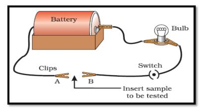
(c) Place the different wires between points A and B one by one and observe whether the bulb glows or not after completing the circuit. It is observed that bulb glows in case of different metals indicating that metals are good conductor of electricity.
