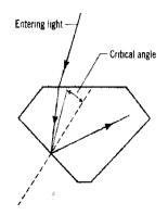
Now consider what happens to the same ray of light within the diamond when the diamond is placed in water. Because water has a larger index of refraction than air, the critical angle increases to 33.3°. Therefore, only this part of the light is reflected back into the diamond, and the remainder escapes into the water. Consequently, less light exits from the top of the diamond, causing it to lose much of its brilliance.
