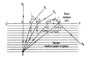
At point D, i> c, and ray, instead of suffering refraction, undergoes reflection totally back along  $DR_4$ , in denser medium. Hence beyond C, rays suffer "Total Internal Reflection.".
