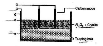
Alumina melts at 200°C. It is a bad conductor of electricity. But when mixed with cryolite and some calcium fluoride, the mixture becomes a good conductor of electricity, and melts at 900-950°C. The iron cell is lined inside with gas carbon which serves as cathode. Carbon rods act as anode. The electrolyte, thus, contains  $Na^+$ ,  $Al^{3+}$ ,  $F^-$  and  $O^{2-}$  ions. On passing electric current,  $Al^{3+}$  ions are discharged at the cathode and the  $O^{2-}$  ions at the anode.
