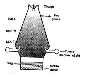
**Function of limestone** Limestone is decomposed to give quicklime.
