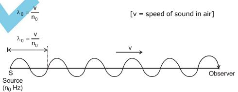
Although sound waves are longitudinal, here we represent sound weaves by the transverse displacement curve as shown in figure to understand the concept in a better way. As source produces waves, these waves travel towards, stationary observer O in the medium (air) with speed v and wavelength  $\lambda_0$ . As observer is at rest here it will observe the same wavelength  $\lambda_0$  is approaching it with speed v so it will listen the frequency n given as
