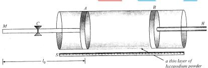
In tube air is filled at room temperature and a thin layer of lycopodium powder is put along the length of the tube. It is a very fine powder particles of which can be displaced by the air particles also. When rod M is gently rubbed with a resin cloth or hit gently, it starts oscillating in fundamental mode as shown in figure, frequency of which can be given as
