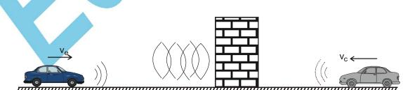
Here we assume that the sound which is reflected by the stationary wall is coming from the image of car which is at the back of it and coming toward it with velocity  $v_c$ . Now the frequency of sound heard by car driver can directly be given as
