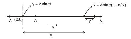
Consider a wave going in the x-direction in a fluid. Suppose that at a time t, the particle at the undistrubed position x suffers a displacement y in the x-direction.
