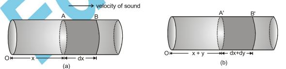
Here we say an elastic wave has propagated along the rod with a velocity determined by the physical properties of the medium. Due to oscillations say a force F is developed at every point of medium which produces a stress in rod and is the cause of strain or propagation of disturbance along the rod. This stress at any cross-sectional area can be given as
