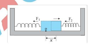
elongated by a length equal to x and that on the right side gets compressed by the same length. The forces acting on the mass are then,  $F_1 = -k \times (\text{force exerted} by the spring on the left side, trying to pull the mass towards the mean position)$
