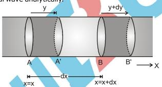
Consider a longitudinal wave propagating in positive x-direction as shown in figure. Figure shows a segmentAB of the medium of width dx. In this medium let a longitudinal wave is propagating whose equation is given as
