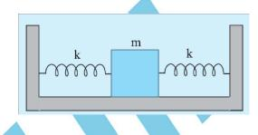
**Ans.** Let the mass be displaced by a small distance x to the right side of the equilibrium position, as shown in Fig. Under thissituation the spring on the left side gets
