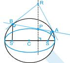
(4) The portion of the tangent to an ellipse between the point of contact & the directrix subtends a right angle at the corresponding focus.
