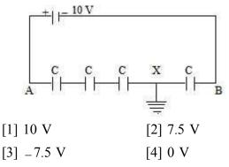
**Sol.** The equivalent capacitance of the circuit is C/4 and the charge on each capacitor is
