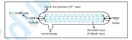
In 1859, **Julius plucker** started the study of conduction of electricity through gases at low pressure in a discharge tube. When a high voltage of the order 10, 000 volts or more was applied across the electrodes, some sort of invisible rays moved from the –ve electrode to the +ve electrode. Since the –ve electrode is referred to as cathode, these rays were called cathode rays.
