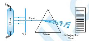
When hydrogen gas at low pressure is taken in the discharge tube and the light emitted on passing electric discharge is examined with a spectroscope, the spectrum obtained is called the emission spectrum of hydrogen.
