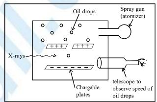
The metal plates were given an electric charge, and as the electric field between the plates was increased, it was possible to make some of the drops travel upwards at the same speed as they were previously falling.
