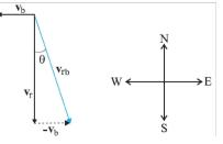
her is the velocity of rain relative to the velocity of the bicycle she is riding. That is vrb =  $v_r \cdot v_b$  This relative velocity vector as shown in Fig. 4.16 makes an angle f'' with the vertical. It is given by
