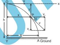
Horizontal component of velocity,  $v_x = u$ Vertical component of velocity,  $v_y = 0 + gt = gt$  $\therefore$  The resultant velocity at point P is
