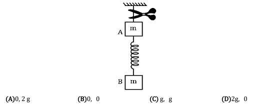
**Q.10** Two blocks A and B of mass M and 2M respectively, are hanging from a ceiling by means of a massless spring and a light string as shown. If the string between the blocks is suddenly cut and the downward acceleration is taken positive, then what will be the acceleration of the block A and B?
