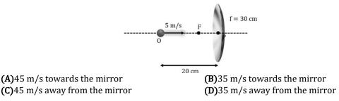
**Q.5** Find the velocity of the image of object O with respect to ground in the given figure. The velocities of the object and the mirror w.r.t ground are given.
