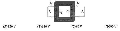
**Q.9** A transformer has 200 turns in primary coil and 600 turns in secondary coil. If a 220 V DC is applied across the primary coil, what will be the voltage across the secondary coil.
