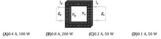
Q.10 In a step-down transformer having primary to secondary turns ratio of 20:1, the input voltage applied is  $250\ V$  and output current is  $8\ A$ . Assuming 100% efficiency, calculate current in the primary coil and the output power.
