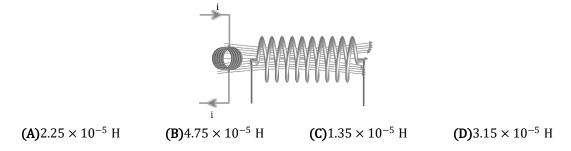
**Q.4** Two coaxial coils are very close to each other and their mutual inductance is**3** H. If a current  $i_1 = 2\sin 30t A$  is passing through the first coil, then find the peak value of induced **emf** in the second coil.
