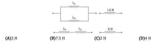
**Q.7** Find the equivalent inductance in the combination given below between points **A** and **B**.
