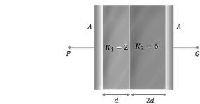
$Q.3 \qquad A \ \text{capacitor} \ \text{is formed by two square metal plates of edge1} \ m, \ \text{separated by a distance1} \ mm. \\ \text{Dielectrics of dielectric constant} \ K_1 \ \text{and} \ K_2 \ \text{are filled in the gap as shown in figure. The new capacitance is}$
