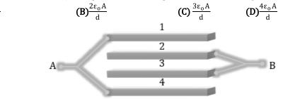
**Q.10** Five similar condenser plates, each of area A are placed at equal distance d apart and are connected to source voltage V as shown in the following diagram. The charge on plates 1 and 4 will be:
