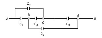
**Q.8** The net capacity between the points A and B in the following circuit will be
