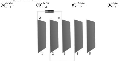
**Q.7** If the two terminals of a battery of 21 V is connected across A and B, the charge flown through the battery will beGiven:  $C_1 = 2 \text{ pF}$ ;  $C_2 = 13 \text{ pF}$ ;  $C_3 = 6 \text{ pF}$ ;  $C_4 = 1 \text{ pF}$ ; and  $C_5 = 12 \text{ pF}$ **(A)**  $5.4 \times 10^{-12} \text{ C}$  **(B)**  $5.4 \times 10^{-13} \text{ C}$  **(C)**  $5.4 \times 10^{-10} \text{ C}$  **(D)**  $5.4 \times 10^{-11} \text{ C}$
