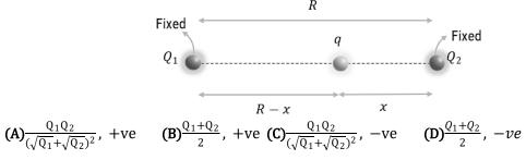
Q.12 In a system of equilibrium of charges, when a charged body (+q) is displaced from its equilibrium position, the net force is [Assume charges +Q to be fixed and consider only axial displacement]
