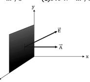
Q.5Find the flux of the electric field through surface ABCD of the inclined plane as shown in figure.<br/>(A)  $E abCos\theta$ (B)  $E abSin\theta$ (C)  $E abTan\theta$ (D)  $E abCot\theta$
