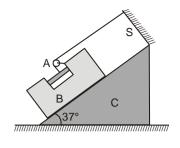
are same. Then the magnitude of acceleration of A is  $\frac{\sqrt{x}}{3}$  m/s<sup>2</sup>. Then x is (sin 37° = 3/5)
