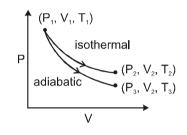
6.\* An ideal gas in a thermally insulated vessel at internal pressure = P<sub>1</sub>, volume = V<sub>1</sub> and absolute temperature = T<sub>1</sub> expands irreversibly against zero external pressure, as shown in the diagram. The final internal pressure, volume and absolute temperature of the gas are P<sub>2</sub>, V<sub>2</sub> and T<sub>2</sub>, respectively. For this expansion, [JEE(Advanced) 2014, 3/120]
