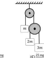
Q.5 Find the acceleration of the block of mass 2m as shown in the figure. (Strings are massless and inextensible)
