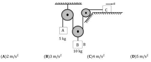
Q.7 In the figure, accelerations of block A, B and C are indicated by a, b and c respectively. Acceleration a, b and c are w.r.t to the ground. Find the acceleration of the body A in terms of b and c with respect to ground if the surface is smooth and pulley and string is ideal.
