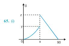
x is the minimum angle of incidence for total internal reflection.
