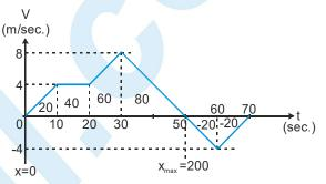
Positive increase in area of v-t curve shows positive increase in displacement. So displacement is increasing till
