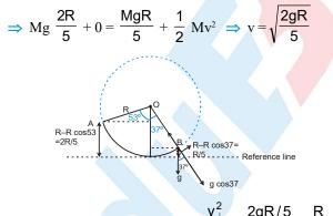
Now, radius of curvature  $r = \frac{v_{\perp}^2}{a_r} = \frac{2gR/5}{gcos37} = \frac{R}{2}$
