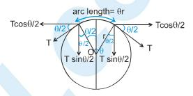
As  $\bullet = 2\pi r$   $\therefore$   $T = m\omega^2 r/2\pi$ Put  $m = 2\pi kg$   $\omega = 10 \pi$  radian/s and r = 0.25 m  $\therefore$  T = 250 N
