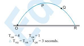
29. From above  $T = \frac{2u\sin\theta}{g} = 4 s$   $\therefore u\sin\theta = 20 \text{ m/s} \implies \text{vertical component is } 20 \text{ m/s}$ for maximum height  $v^2 = u^2 + 2as \implies 0^2 = 20^2 - 2 \times 10 \times s \text{ s} = 20 \text{ m}.$
