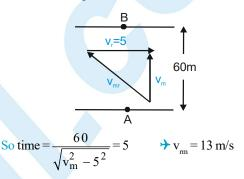
27. For shortest time then maximum velocity is in the direction of displacement.
