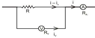
$$\text{measured resistance} = \frac{v}{i} = \frac{i R R_v / (R + R_v)}{i}$$
