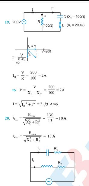
Power dissipated =  $i_{1rms}^2 R_1 + i_{2rms}^2 R_2 = 10^2 \times 5 + 13^2 \times 6$
