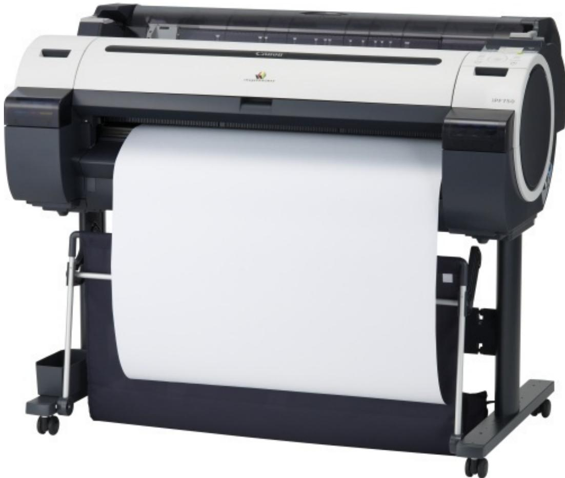
Plotters can automatically change their pens and so can produce colour output. The lines drawn by a plotter are continuous and very accurate. Plotters are very slow but produce high quality output. The quality of the output produced by ink jet printers is now very good and large format (big) ink-jet printers are steadily replacing plotters for most tasks.
