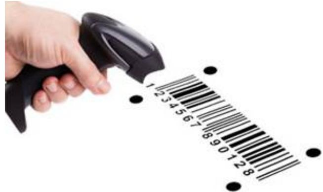
Bar Code Reader scans a bar code image, converts it into an alphanumeric value, which is then fed to the computer to which bar code reader is connected.
