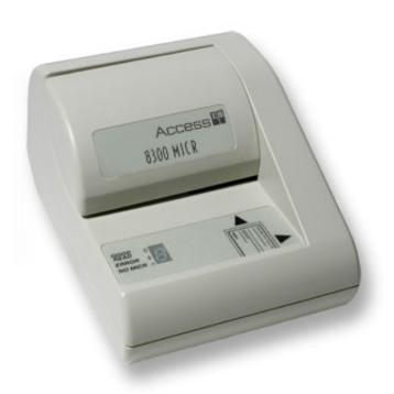
MICR readers can only read one special font which can represent only numbers and a few punctuation marks. They can read characters very quickly and with 100% accuracy. Information printed in magnetic ink is also very secure. It is not possible to change the information by writing over it with a pen and the printed numbers are not damaged by folding (as often happens with cheques). Both the reader used by MICR and the special ink are expensive.
