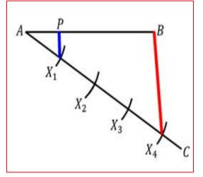
**Step2**: Draw a segment BD of any convenient length making the same angle with AB as AC on the opposite side of AC.
