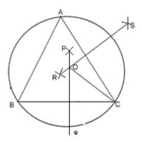
Step 1: A triangle ABC is constructed with BC = a, CA = b and AB = c.
