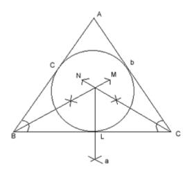
**Step 1**: Triangle ABC in which BC = a, CA = b and AB = c is constructed.
