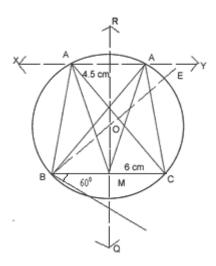
Step 1: BC = 6cm is drawn and  $\angle CBP = 60^{\circ}$  is made downwards with BC of any length.
