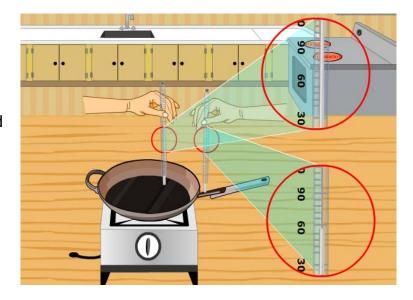
We observe that temperature of metal part increases rapidly, whereas temperature of handle of plastic part remain same or slightly change. Thus, we conclude that plastic is a poor conductor of heat. So it is used to make a handle of utensils.
