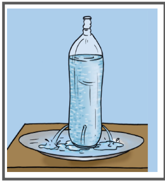
Liquids exert equal pressure at the same depth
