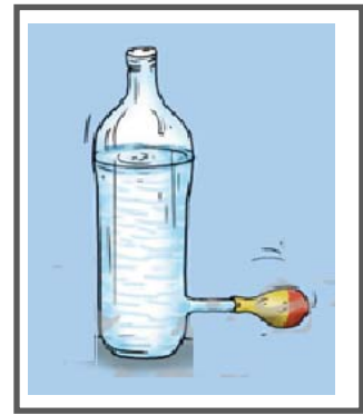
Pressure exerted by water at the bottom of the container depends on the height of its column.
