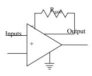
The difference amplifier above has a drawback that it draws a significant current from the inputs. It turns out that a difference amplifier with high input impedance requires at least 3 op-amps. Such circuits are commonly packaged into a single chip called an instrumentation amplifier. The output is given by  $V_0=G(V_+-V_-)$ , where the gain G is set using an external resistor. Instrumentation amplifiers are useful for measuring small voltages because they cancel common-mode noise.
