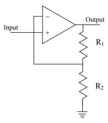
The next circuit is an non-inverting amplifier. The voltage on the "-" terminal must be equal to the input voltage, therefore the output voltage  $V_0 = (1+R_1/R_2)$  V<sub>i</sub>. This circuit has a gain  $\geq 1$ . Its input impedance is equal to the input impedance of the op-amp, typically in the  $G\Omega$  range, and it draws virtually no current from the input.
