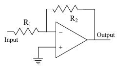
The circuit on the left is an inverting amplifier. Its analysis proceeds as follows. Suppose a voltage  $V_i$  is applied to the input. Since the "+" input of the op-amp is at ground, the "-" input must also be at zero voltage following the first op-amp rule. Therefore the current flowing through resistor  $R_1$  is  $I = V_i/R_1$ . The current going into the amplifier input is zero, therefore the same current I must flow through the
