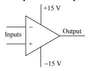
Operational amplifiers (op-amps) are the simplest and most commonly used analog integrated circuit. The circuit basically amplifies the voltage difference between the two inputs by a very large factor,  $10^6$   $-10^7$ . Op-amps typically require  $\pm 15$  V power supplies, but can run almost as well with any supply voltage between  $\pm 5$ V and  $\pm 20$ V. In circuit diagrams the power supply lines are usually not shown explicitly.
