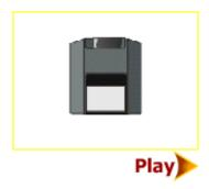
The Zip Drive uses a disk or cartridge just slightly larger than a 3.5 inch floppy but capable of storing 100 MB of data!
