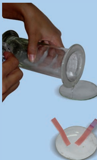
Fig. 4.4 (b) : Testing of solution with litmus papers
