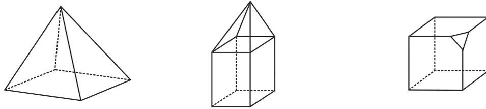
Each of these solids is made up of polygonal regions which are called its **faces**; these faces meet at **edges** which are line segments; and the edges meet at vertices which are **points**. Such solids are called **polyhedrons**.
