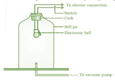
After some time when less air is left inside the bell jar you will hear a very feeble sound. At the end, when all the air is removed completely, we will not be able to hear the sound of bell. This show sound requires material medium.
