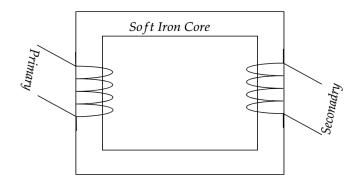
The transformer work on the principle of the mutual induction that is whenever a current is associated with the primary coil charges then an emf is induced in the secondary coil. Hence when a transformer in which the output that is the secondary voltage is greater than its induce or primary voltage it is known as step up transformer.
