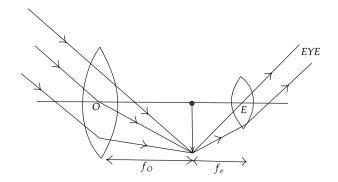
Here, fO is the focal length of the objective lens and fe is the focal length of the eyepiece lens.
