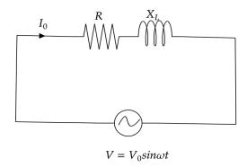
The given circuit show that the resistor and the inductor are connected in series.
