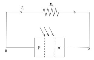
The construction of a silicon solar cell is usually made up of thick layer of n-type semiconductor which is layered by a thin layer of p-type semiconductor. Then the electrodes are placed on the top of the p-type semiconductor and then another electrode for collecting current is attached to the bottom of the n-type semiconductor.
