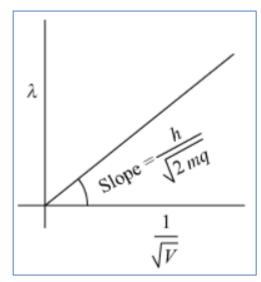
The slope of the graph is  $\frac{h}{\sqrt{2mq}}$  considering we know slope and mass of the charged particle
