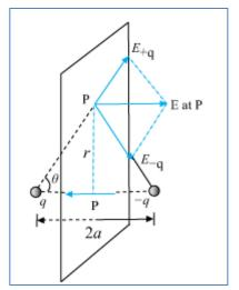
The magnitude of the electric field due to two charges +q and -q are
