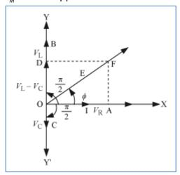
As the inductor, capacitor and the resistor are connected in series so the current through all of them is same (same amplitude and same phase) Let the current be 1= Im sin w t The voltage across each component has a different phase relation with the current.
