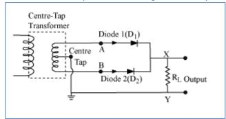
When the voltage at A with respect to the center tap is positive, and the voltage at B is negative. Then, Di is forward biased and D2 is reversed biased. Hence, Di conducts and D2 does not. When the voltage of A becomes negative, then B becomes i-ve. Therefore, Di does not conduct and D2 conducts. Hence, we obtain output voltage during both the positive as well as negative half of the cycle.
