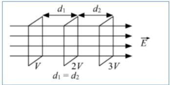
Difference: For constant electric field, the equipotential surfaces are equidistant for the same potential difference between these surfaces; while for increasing electric field, the separation between these surfaces decreases, in the direction of the increasing field, for the same potential difference between them.
