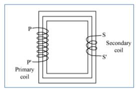
Working Principle: A transformer works on the principle of electromagnetic induction.
