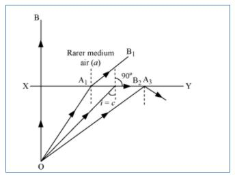
Total internal reflection is the phenomenon of reflection of light into a denser medium from an interface of the denser medium and the rarer medium. Two essential conditions for total internal reflection: Incident ray should travel in the denser medium and refracted ray should travel in the rarer medium.
