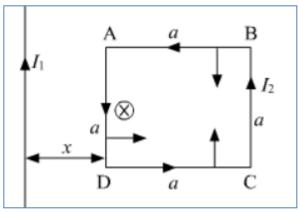
According to the right hand screw rule, the magnetic field will be into the plane across the loop Force on length AD
