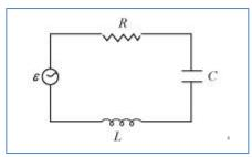
An AC source E with voltage  $v = v_m \sin \omega t$  is applied across LCR circuit
