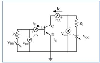
Variation of collector current  $I_c$  with the collector emitter voltage  $V_{\it CE}$  is called output characteristic.
