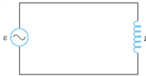
An ac source connected to an inductor.
