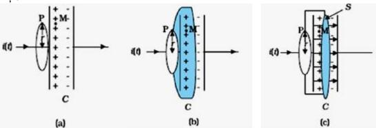
Applying ampere's circuital law to fig (a) we see that, during charging, the right hand side in Ampere's circuital law equals  $\mu_0 I$
