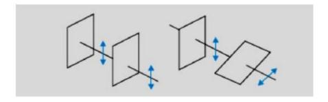
Light from the sodium lamp passing through the single Polaroid sheet ( $P_1$ ) does not show any variation in intensity when this sheet is rotated.
