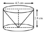
Given Height (b) of the conical Part = Height (h) of the cylindrical part = 2.8 cm Diameter of the cylindrical part = Diameter of the conical part = 4.2 cm  $\therefore$  Radius  $\rightarrow$  of the cylindrical part = Radius  $\rightarrow$  of the conical part = 2.1 cm Slant height (I) of the conical part =  $\sqrt{r^2 + h^2}$
