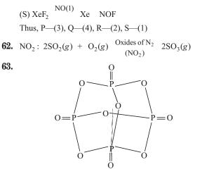
Here four oxygen atoms are bonded to each phosphorus atom.
