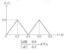
Induced emf in the coil due to change in magnetic flux passing through it,  $e = \left| \frac{d\phi}{dt} \right| = NA \left| \frac{dB}{dt} \right|$
