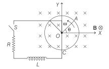
without friction along a fixed conducting circular ring in the same plane as that of rotation. A uniform and constant magnetic induction **B** is applied perpendicular and into the plane of rotation as shown in figure. An inductor L and an external resistance R are connected through a switch Sbetween the point O and a point C on the ring to form an electrical circuit. Neglect the resistance of the ring and the rod. Initially, the switch is open. (1995, 10M)
