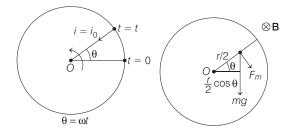
The steady state current will be  $i = i_0 = \frac{B\omega r^2}{2R}$
