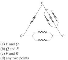
**16.** The effective resistance between points P and Q of the electrical circuit shown in the figure is (2002, 2M)
