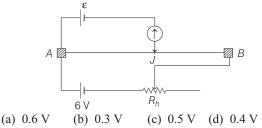
**10.** A potentiometer wire *AB* having length *L* and resistance 12r is joined to a cell *D* of EMF  $\varepsilon$  and internal resistance *r*. A cell *C* having emf $\frac{\varepsilon}{2}$  and internal resistance 3r is connected. The length *AJ* at which the galvanometer as shown in figure shows no
