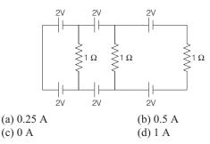
**13.** In the circuit shown below, the current in the  $1\Omega$  resistor is
