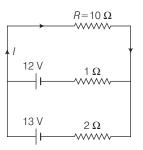
$$E_{eq} = \frac{\Sigma E / r}{\Sigma (1 / r)} = \frac{\frac{12}{1} + \frac{13}{2}}{\frac{1}{1} + \frac{1}{2}} = \frac{37}{3} V$$
