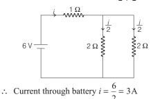
This current is equally distributed in  $2\Omega$  and  $2\Omega$ resistances. Therefore, the desired current is  $\frac{i}{2}$  or 1.5 A.
