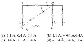
**8.** In the given circuit, the cells have zero internal resistance. The currents (in Ampere) passing through resistances  $R_1$  and  $R_2$  respectively are (2019 Main, 10 Jan I)
