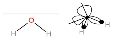
Hydrogen peroxide has a non-planar structure both in gas and solid phase. The dihedral angle in gas and solid phase is 111.5° and 90.2° respectively. The structure can be shown as:
