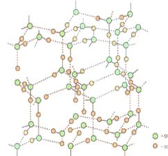
The structure is highly ordered and has hydrogen bonding. Each oxygen atom is surrounded tetrahedrally by four other oxygen atoms at a distance of 276 pm. The structure also contains wide holes that can hold molecules of appropriate sizes interstitially.
