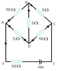
**Ans:** Current flowing through various branches of the circuit is represented in the given figure.
