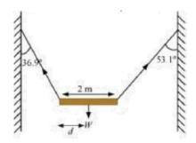
**Ans:** The free body diagram of the bar can be drawn as shown in figure.
