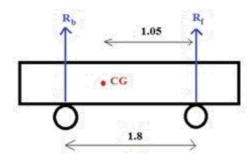
The forces in the figure,  $R_f$  and  $R_b$  are the forces exerted by the level ground on the front wheels and back wheels respectively.
