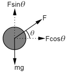
The vertical component of this applied force acts upward. This reduces the effective weight of the mower.
