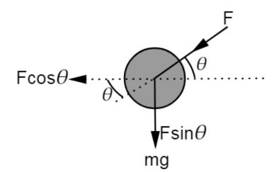
In this case, the vertical component of the applied force acts in the direction of the weight of the mower. This increases the effective weight of the mower.
