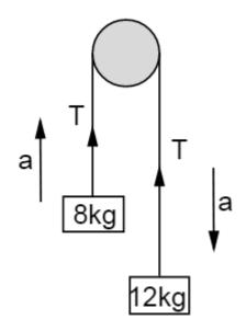
Smaller mass,  $m_1 = 8kg$ Larger mass,  $m_2 = 12kg$ Tension in the string = T Mass  $m_2$ , owing to its weight, moves downward with acceleration a, and mass moves  $m_1$  upward.
